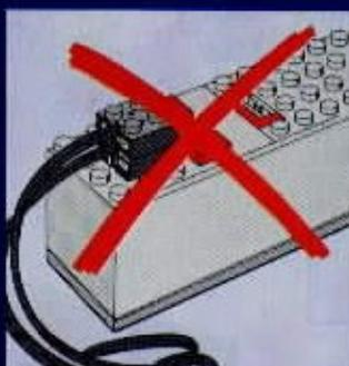
Never snap the wire back onto itself. Should a short circuit occur, the current is automatically cut out until the fault has been corrected.
